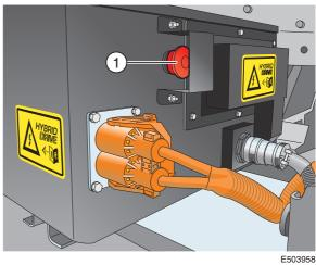
In case it is not possible to enter the cab and disconnect the vehicle batteries (24V), push the red service switch (1) on the hybrid battery box.
